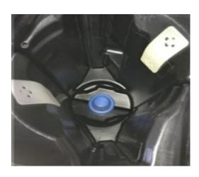
Custom urethane plug engineered to absorb the vibration.
