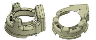
TPU hold down piece designed to protect wires on the stators and hold down the parts during transit.
