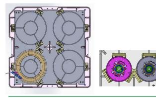
Generic base tray to accommodate multiple varieties of stator and rotor parts.
